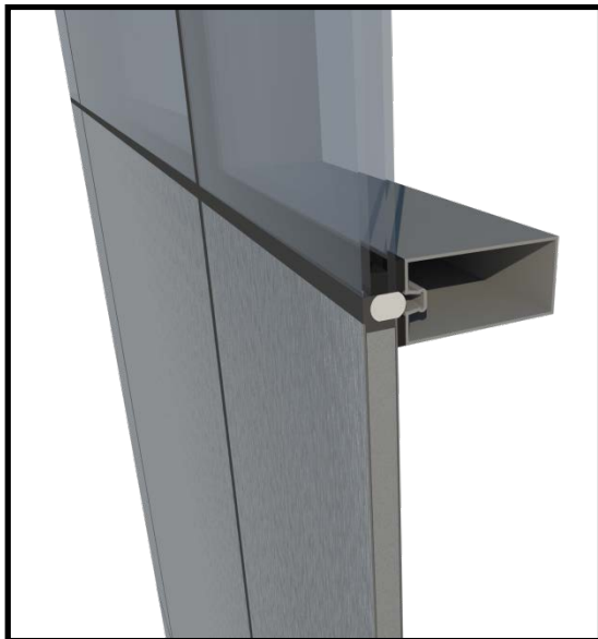
Figure 3: Enlarged view of structural silicone attachment of glass and spandrel to curtain wall frame.
