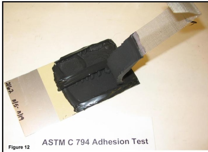
Figure 12 – 1 in. screen mesh embedded in sealant on metal coupon. Figure 13 – Test specimen mounted in Instron for 180° pull.
