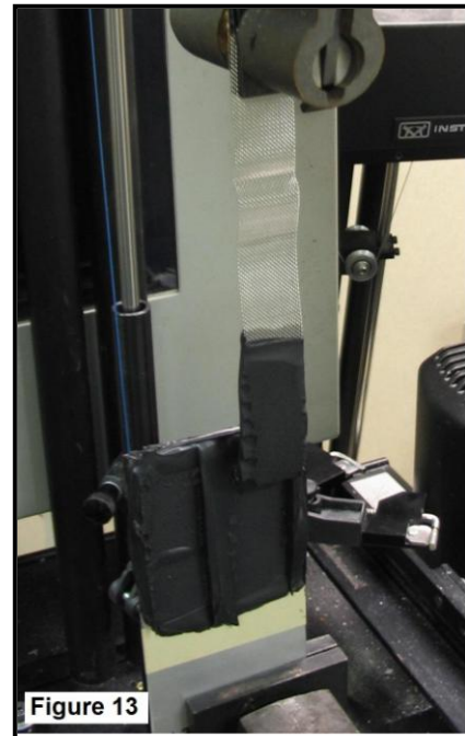
Figure 12 – 1 in. screen mesh embedded in sealant on metal coupon. Figure 13 – Test specimen mounted in Instron for 180° pull.
