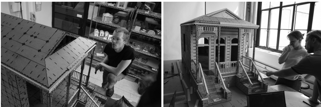
Figure 11 a rough prototype from the construction model and a partially finished prototype from a corrected construction model
