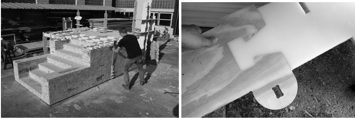
Figure 10 Digital mockup of one section with OSB board and detail mockup of micro tool paths
