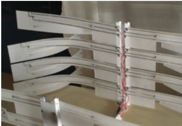
Figure 13. View of operational model showing activation of fins and fin and mast circuitry.
