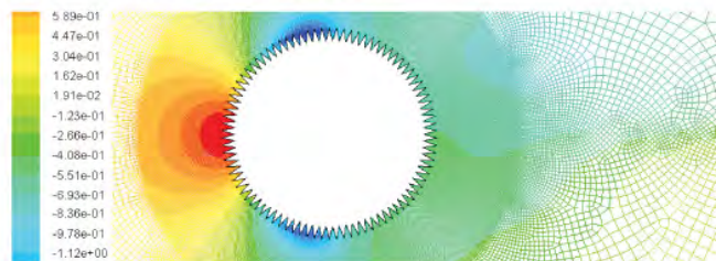
V-shaped protrusions of Saguaro Cactus CFD analysis - LT Alberfi (2005)
