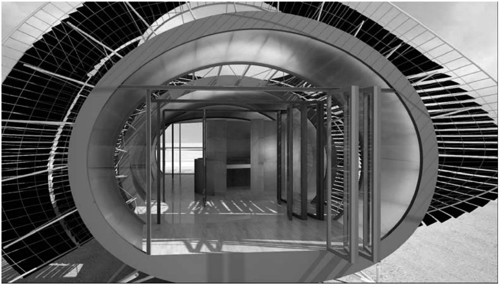
Figure 5: Exterior view of early Design Development phase multilayered envelope with doubly curved shell
