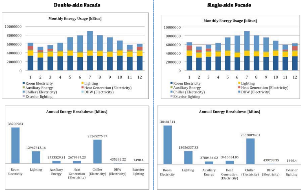
Figure 7. Double skin façade energy simulation results (Left side) Single skin façade energy simulation results (Right side)
