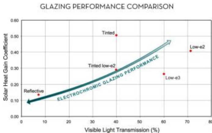
FIGURE 2: Graph of visible light transmission ( T_{vis} ) versus solar heat gain coefficient (SHGC) which demonstrates the heat gain and light transmission range of a high performance EC product compared with examples of standard static glass.
